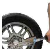
Completion of tightening process with Blue signal.
