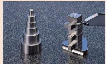
Using a base, plain jaws, tie rods, flat head screws and gauge blocks, a gage was constructed to enable rapid comparison measurement of a stepped workpiece. (Sample workpiece)
