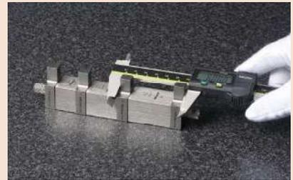
Using plain jaws, tie rods, knurled head screws and gauge blocks, a gage was constructed to enable rapid comparison measurement of a stepped workpiece. (Sample workpiece)
