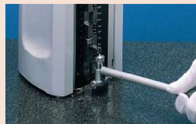
Bore gage zero-setting
