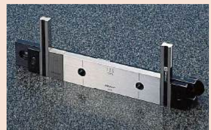
Use of B-type connectors in gage construction
