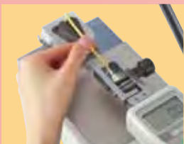
Put a terminal on a hook.
