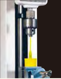
Resin molding tension exception strength test with GC-5.
