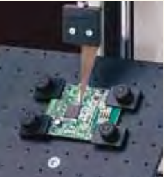
Chip components solder joints shear strength test
