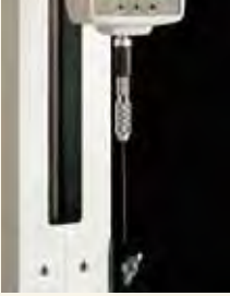
Wire tension strength test with CP-150N
