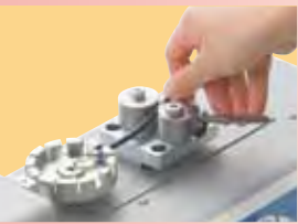
Hook for a terminals, and grip a wire.
