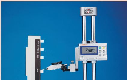
Checking accuracy of height gage
