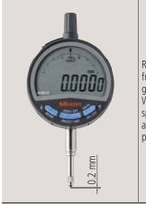
Repeatability in the range of 0.2 mm from the lowest rest point is not guaranteed for Digimatic indicators. When setting the origin or presetting a specific value, be sure to lift the spindle at least 0.2 mm from the lowest rest
