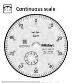
Graduation: 0.001 mm, **2110A-10** Measuring range: 1 mm Double scale spacing
