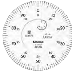
Graduation: 0.01 mm, 3050A Measuring range: 20 mm
