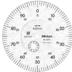
Graduation: 0.01 mm, 3046A Measuring range: 10 mm
